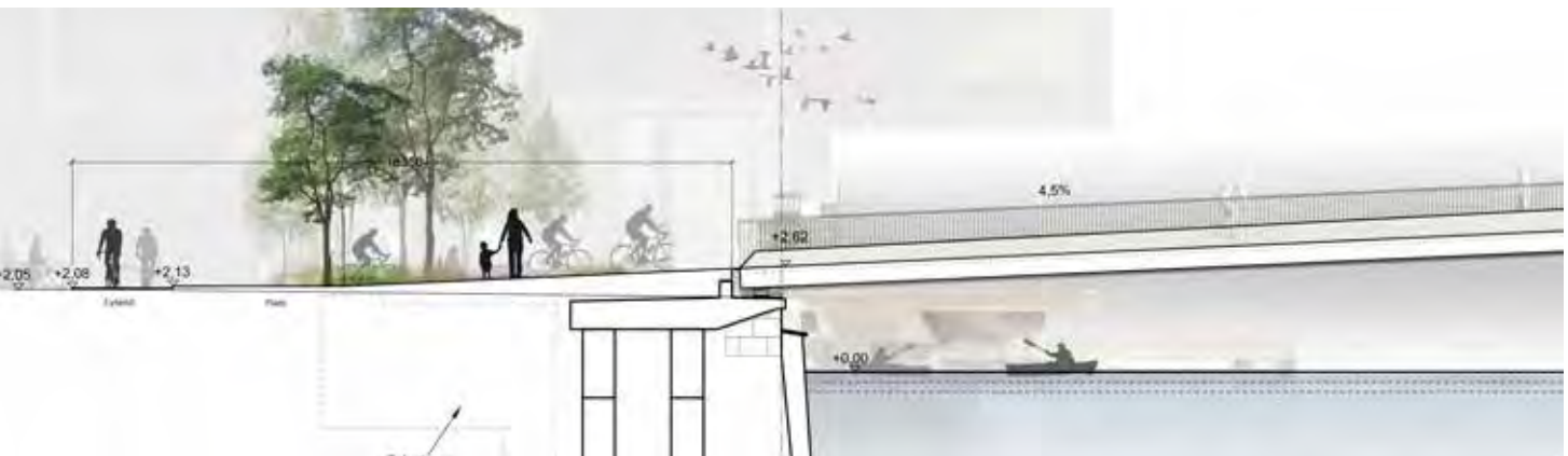
Section of western bridge abutment
